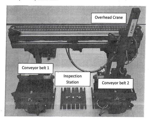
The system is composed by an overhead crane, two conveyor belts and an inspection station. Each conveyor has a presence sensor that has the logic value TRUE, or 1, when a part is detected and FALSE, or 0, otherwise. The inspection station has also one such sensor. Parts cannot be placed in the inspection station or in conveyor belt 2 if they are already occupied.
