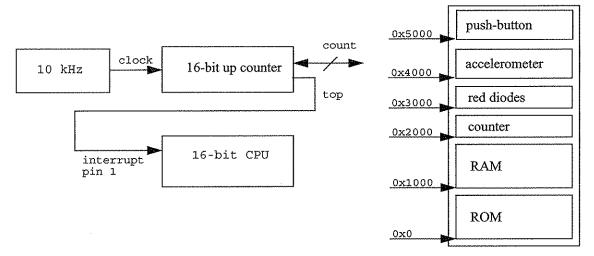
When the push-button is pressed a logic one is present at address 0x5000 (else logic zero).
