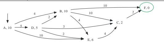
Above is given a graph, with weights on the edges, and for each node an estimate of the cost to reach the goal node F.
