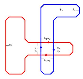
consider the local plant models  $P_1$  and  $P_2$  which model the states between the events  $a_1 - a_5$  and  $b_1 - b_6$ .
