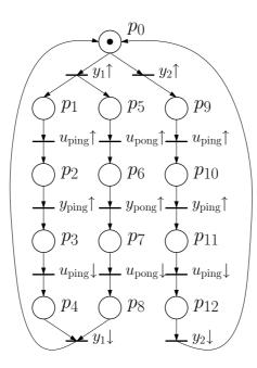
a) Draw a Sequential Function Chart implementing the controller. Collapse the places in request/answer pairs (e.g. collapse  $p_1$  with  $p_2$ , and  $p_3$  with  $p_4$ ).
