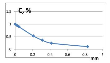
b) Define on the sketch the thickness of the carburized layer. Calculate, at the same conditions, what time is required to double the carburization depth. (2p).
