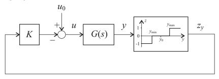
If K is too large the system will exhibit self-oscillations. Determine a value of K that should probably not be exceeded!
