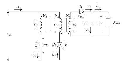
For CCM and DCM operation with no current in winding N<sub>2</sub>, derive the relationship between the output and input voltage (in terms of switching frequency  $f_{sw}$ , duty cycle *D*, mutual inductance  $L_m$  and load resistance  $R_{load}$ ).
