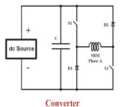
Fig Q4-2: Drive for one phase of an SRM
