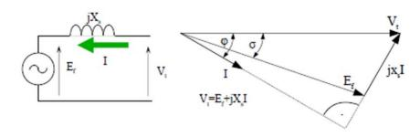
*Proble 7*:Since a PM motor is magnetized by its permanent magnets, no magnetixing current is needed. Hence, the power factor of a PM motor is higher. As a result, the same current magnitude will generate a higher power in a PM motor compared to a IM.
