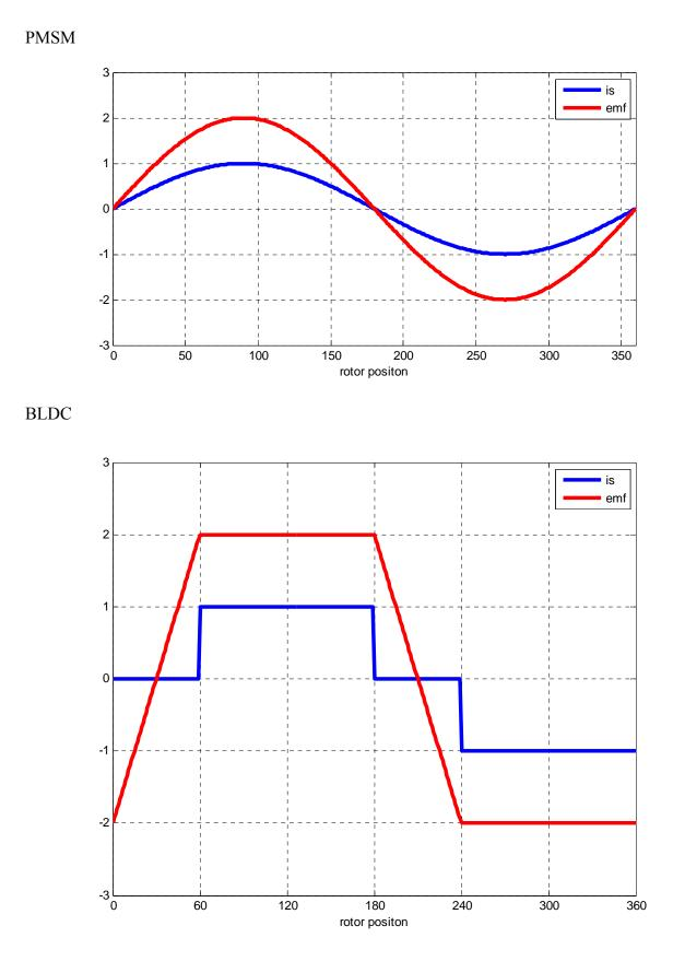
b) In order to have produce a constant torque the current in each phase is controlled to be constant during the time period when the emf is constant. As a result, the current will flow
