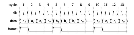
Frame signals start of new serial frame (in this case 4 words) Flow control can be at frame granularity or word granularity
