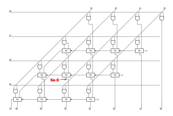
B0=0, B1=0, B2=1 and A0=0, A1=0, A2=1 are inputs that will activate the fault (the sum of the FA will be "1" which is the opposite value from the stuck-at-0)
