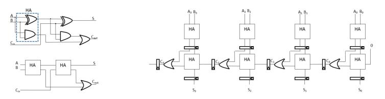
The total number of stages are 5. Then, the delay of each stage is 0.5+2+0.5=3ns, the total latency of the pipelined adder is 5\*3=15 ns, and its throughput is 1/3 results/ns.
