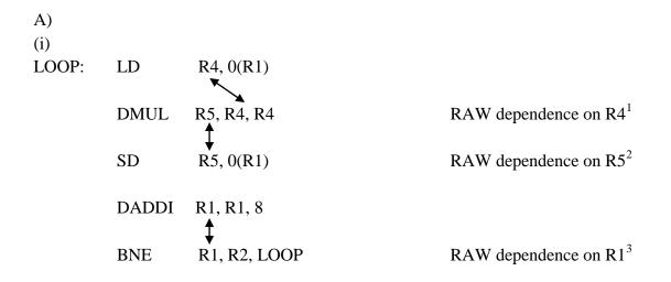
Assuming a 5-stage pipeline structure using forwarding/bypass for handling of RAW hazards (shown as red thick arrows):
